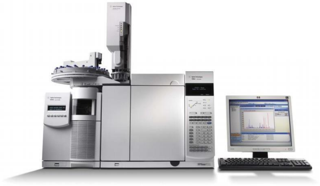
Figure 16. Agilent Technologies 7890A Gas Chromatograph coupled with a Mass Selective Detector (MSD), 5975C (Agilent Technologies).
